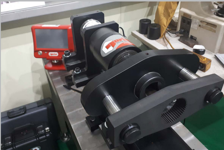
Norbar designed and manufactured Power Tool Test Rig for verifying Norbar Power Tools
